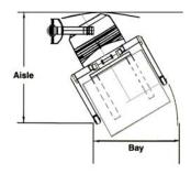
Note: Aisle dimensions listed assume the bay width to be straddle OD plus 2" (1" on each either side of straddle leg).
